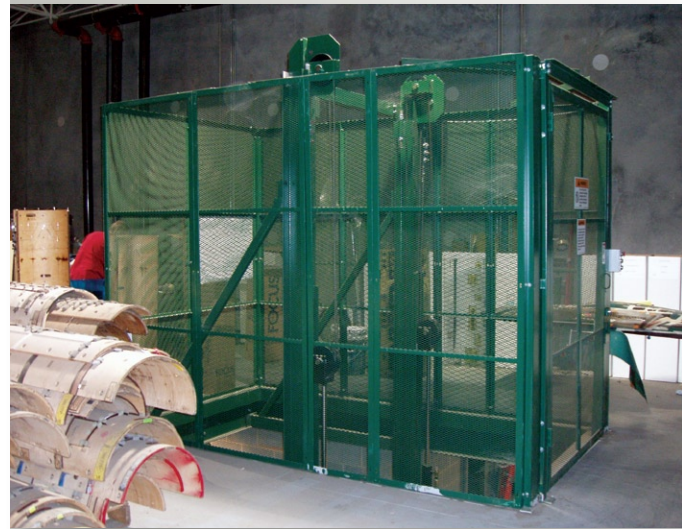
Wildeck's VRC saves time and safely transports dies to the production area.
