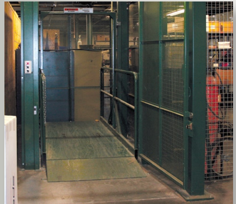
Wildeck's VRC saves time and safely transports dies to the production area.
